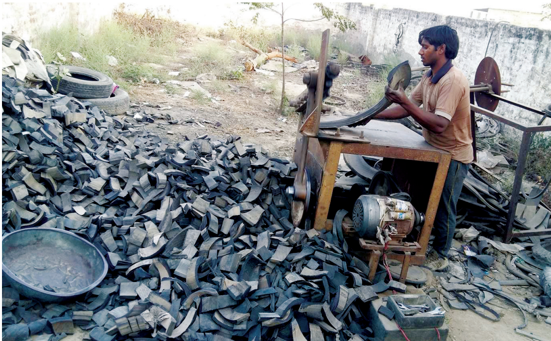
Photo 4: Kohlu or Kalesar being operated to manually shred waste rubber for burning
