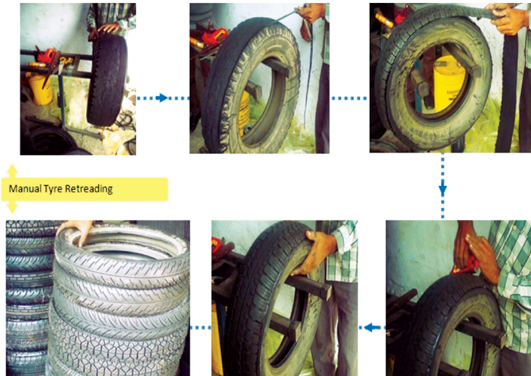
Photo 3: Manual Retreading of a Tyre in Meerut
